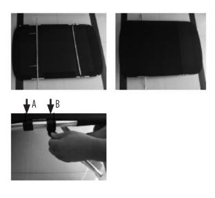
Step 5: Install the bimini top under the top section of your wakeboard tower. Install the four bimini rings on the tower's bars as shown in the right pictures, but don't tighten the bolts of the rings.
