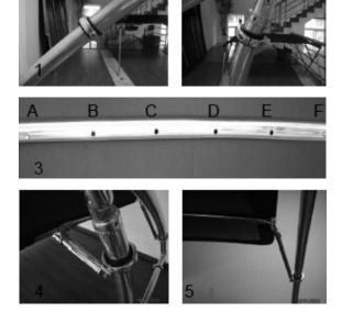
Step 6: Install the bimini top above on the tower. Mount two rings on the front bars of tower, and mount two rings on the top section as shown in the right pictures, but don't tighten the bolts of the rings.
